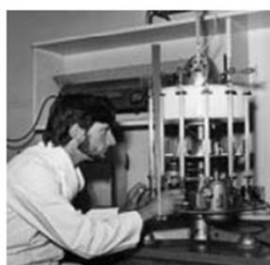
Measuring O 2 uptake using a Warburg apparatus – 10 ml incubations
